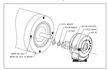
Rotate the tether arm until it is at the correct orientation and is aligned with the mounting holes on the the motor or equipment. Install one steel washer on both sides of the nylon washer. Refer figure above. Fasten the tether arm to the motor or machine housing using the supplied 3/8" bolt (4.5" C-face applications) or 1/2" bolt (8.5" C-face applications). Ensure that there is no stress or flexing of the tether arm when secured.
