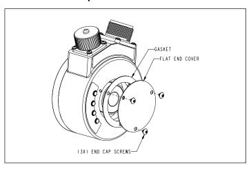
The encoder ships with an endcap to cover the back end of the encoder body and, although optional, it is recommended for additional environmental protection. To install, remove the factory installed three screws at the back of the encoder, properly discard the removed back plate and the three screws. Unpack the endcap, gasket and the three screws from the factory supplied kit. Align the three holes and fasten the gasket and end cap to the encoder body as shown.
