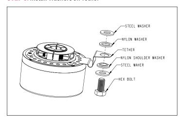
Slide the flat nylon washer on the side away from the bend and the flanged nylon washer on the side of the bend and press them together until they are fully seated in the tether hole. One steel washer is to be used on each side of the nylon washer.
