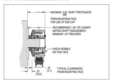
Follow the 3 step installation check to ensure a good installation thus far. Refer to figure above for key reference dimensions
