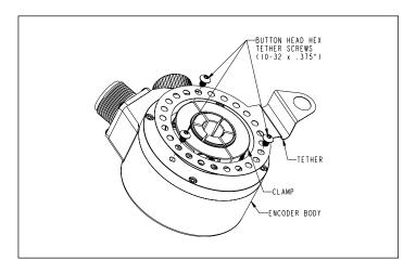
Rotate the tether to the required orientation and tighten the tether arm to the encoder body using the three screws provided. The hollowshaft series encoder tethers can be rotated in 15 degree increments so that connector or cable exit can be conveniently located.
