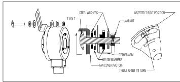
Slide and insert the T-bolt as shown in the figure into the fan cover. Use the supplied insulating hardware and washers as shown. Tighten the jamnut to firmly secure the tether.
